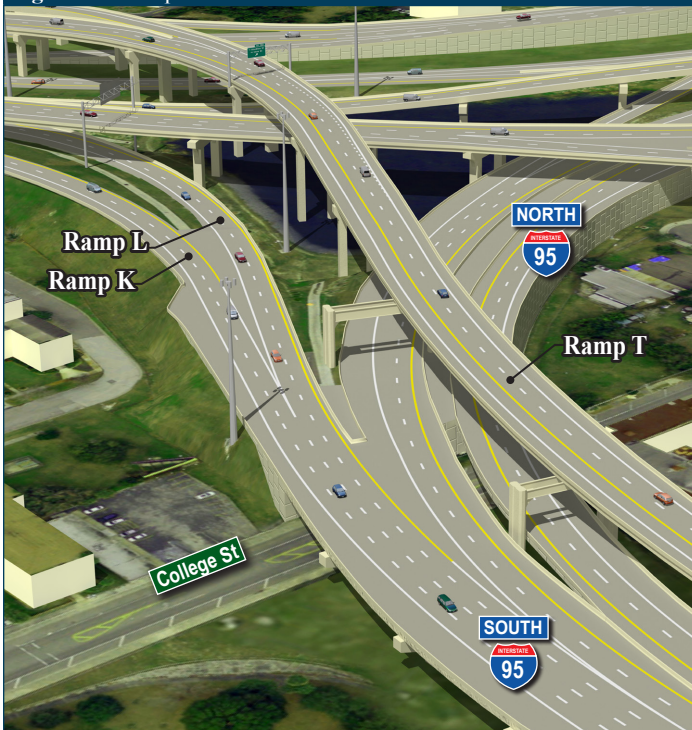
Figure 2 – Ramp T Solution
